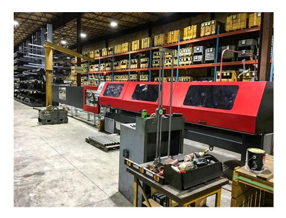
New automatic CNC cutting Line Mod. NEW LINE 350 for 90° cuts, suitable for cutting hollow or solid bars with round, square or rectangular sections, featuring automatic loading and unloading of pieces. The "CI" type automatic loader with inclined worktable is designed for loading hollow bars with round, square or rectangular sections; rapid centralized adjustment of bar dimensions by means of just two handwheels.
